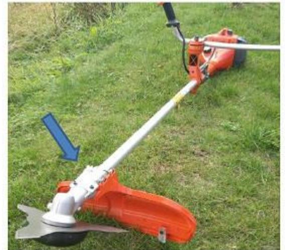
Protective guard fitted correctly
