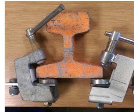
Approved clamp shown on left, non-compliant, ill-fitting clamp on right
